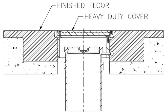
**Z1400 "LEVEL TROL" FLOOR CLEANOUT Exploded Parts List and Replacement Parts**
