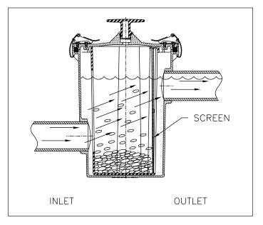
**Note:** Damage from high-temperature water will not occur to the acid resistant composite material of this unit when installed downstream from a dishwasher. There is a chance, however, that the thin-walled PVC screen in the bucket may deform. It is recommended that a stainless steel perforated screen be used in applications that involve high-temperature water.
