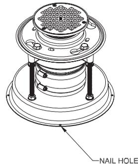
**Note:** Some localities' building codes do not allow a shielded coupling or rubber gasket to be buried in concrete. For applications such as this, a section of 6" PVC pipe can be used to act as a barrier to keep concrete from coming in contact with the rubber materials.
