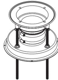
**Step 6** Trim the studs down so they are flush with the bottom of the plate. Set the assembly onto a level surface and check to ensure that the drain body is level with the plate. The flanged nuts can be loosened and tightened to allow for any necessary adjustments. Once leveled, trim any studs that extend beyond the cavity of the plate.
