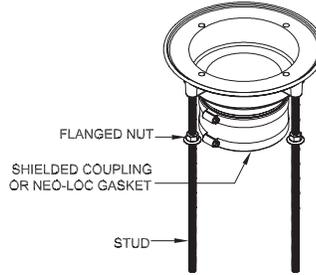
**Step 4** Insert the studs through the four holes of the plate with the plate cavity facing downward. Set the drain body at the required rough-in height and screw the flanged nuts down until they are flush against the top of the plate.
