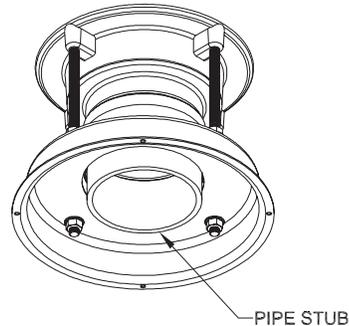
**Step 8** Once the assembly is complete and set at the proper rough-in height, place the assembly in the proper location prior to concrete pour. The assembly can be nailed down to the concrete forms by using the nail holes provided on the rim of the plate.
