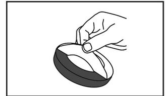
2. Carefully lift and remove adhesive backing off one side of NEO-SEAL gasket.
