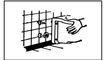
6. Place closet in position over adjustable coupling without delay. Coupling should extend beyond finished wall far enough to compress NEO-SEAL gasket (see other side).
