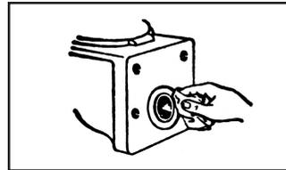
1. Wipe gasket recess of fixture clean with dry cloth. Remove and discard inner foam circle from NEO-SEAL gasket.
