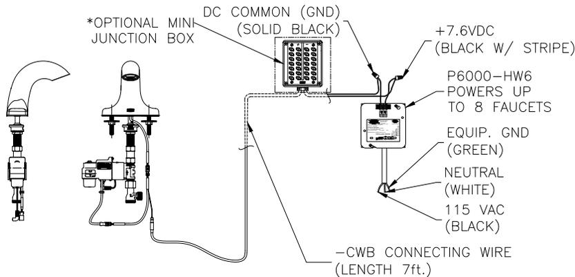
OPTIONAL: \* P6000-MJ mini junction box streamlines wiring for connecting up to 8 faucets to the P6000-HW6 power converter.
