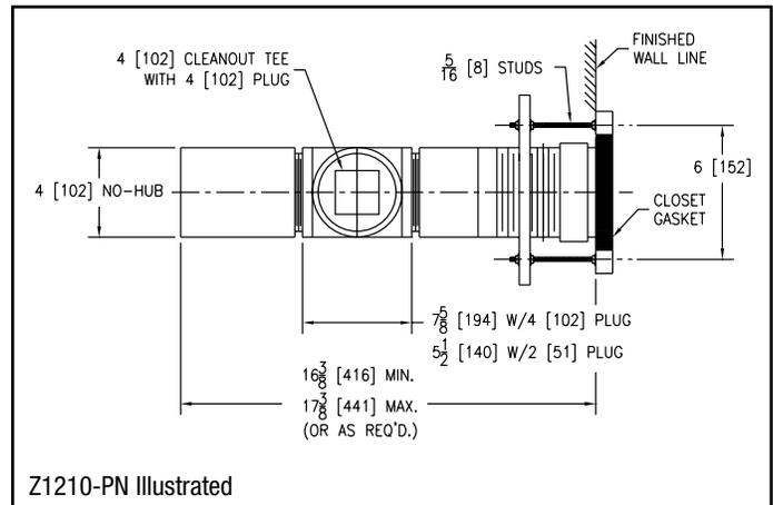
**-PC** Coupling Connection with 4" [102mm] Cleanout for Penal Fixtures (Z1214 and Z1215)
