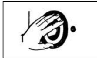
3. Press adhesive-coated side of NEOSEAL gasket firmly into gasket recess in fixture being sure it bottoms out in groove, and that contact between adhesive and china is maintained.
