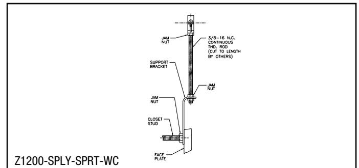
**Water Closet Carriers Z1203, Z1204, Z1207, Z1208, Z1209, Z1212, Z1214, Z1215, Z1216, Z1280, Z1282, Z1283, Z1284 and Z1285**
