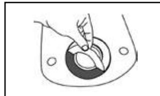
5. Remove adhesive backing off other side of NEO-SEAL gasket.
