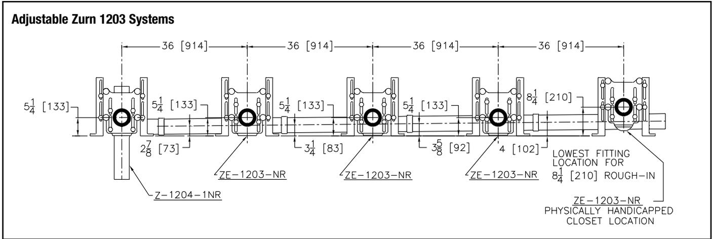
For installation of fixtures, up to a ten fixture maximum, either side of stack fitting:
