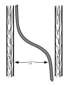
Since Zurn PEX tubing expands or contracts 1" for every 100' of pipe for every 10° of temperature change, you must allow for expansion and contraction in long runs with a 12" horizontal offset.
