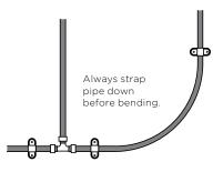
Zurn PEX straps and hangers hold pipe in position and prevent strain on fittings when the pipe is bent.
