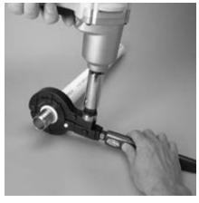
6 Checking – Check crimp using the supplied "GO Gauge."
