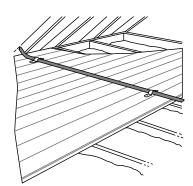
Straps can be as far as 6' apart if the pipe is continuously supported.
