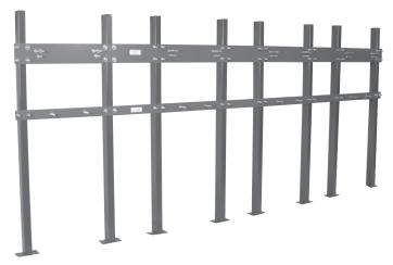
Multiple station plate system provides an extended length plate fabricated with exact center-to-center locations to accommodate a bank of multiple urinals. Custom-length plates are specific to job requirements and are provided with loose uprights and boxed mounting hardware and studs. Ideally suited for prefabricated applications.
