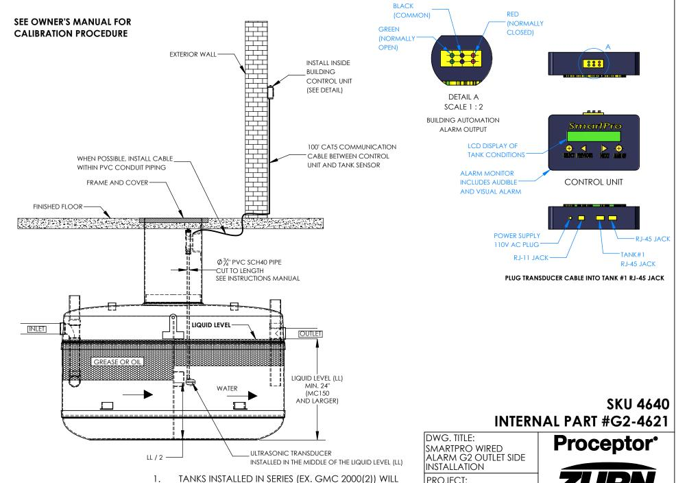
ALARM IS SHOWN TO BE INSTALLED ON OUTLET SIDE OF TANK
