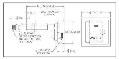
**ENGINEERING SPECIFICATION:** ZURN Z1320 Encased Ecolotrol anti-siphon, automatic draining wall hydrant for flush installation. Complete with copper casing, all bronze interior parts with one-half turn ceramic disc cartridge and combination 3/4" [19 mm] female solder and 3/4" [19 mm] male pipe thread inlet. Stainless steel box and hinged cover with operating key lock and "WATER" stamped on cover. (All solder connections are lead free.)
