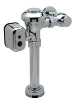
adjusts to its environment at power up and is powered by a 7.6 VDC power converter. Each power converter can accomodate up to eight flush valves. The valve is complete with high back pressure vacuum breaker, one piece hex coupling nut, adjustable tailpiece, spud coupling and flange for top spud connection. Control stop has internal siphonguard protection, vandal resistant stop cap, sweat solder kit, and a cast wall flange with setscrew. Internal seals are made of chloramine resistant materials.
