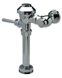
back pressure vacuum breaker, one-piece hex coupling nut, adjustable tailpiece, spud coupling, and flange for top spud connection. Control stop has internal siphonguard protection, vandal-resistant stop cap, sweat solder kit, and a cast wall flange with setscrew. Internal seals are made of chloramine resistant materials.
