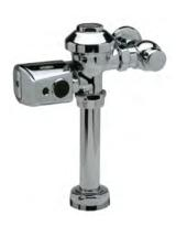
polycarbonate housing and chrome-plated metal cover with manual override push button, high back pressure vacuum breaker, one-piece hex coupling nut, adjustable tailpiece, spud coupling and flange for top spud connection. Control stop has internal siphon-guard protection, vandal-resistant stop cap, sweat solder kit, and a cast wall flange with setscrew. Internal seals are made of chloramine resistant materials.
