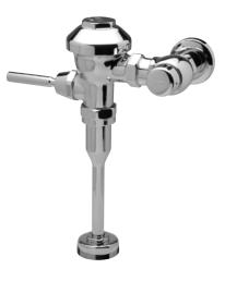
back pressure vacuum breaker, one-piece hex coupling nut, adjustable tailpiece, spud coupling, and flange for top spud connection. Control stop has internal siphonguard protection, vandal-resistant stop cap, sweat solder kit, and a cast wall flange with setscrew. Internal seals are made of chloramine resistant materials.
