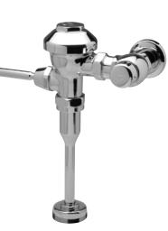
back pressure vacuum breaker, one-piece hex coupling nut, adjustable tailpiece, spud coupling, and flange for top spud connection. Control stop has internal siphonguard protection, vandal-resistant stop cap, sweat solder kit, and a cast wall flange with setscrew. Internal seals are made of chloramine resistant materials.
