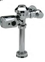
actuator, a battery powered automatic sensor, high impact resistant polycarbonate housing and chrome-plated metal cover with manual override push button, high back pressure vacuum breaker, one-piece hex coupling nut, adjustable tailpiece, spud coupling and flange for top spud connection. Control stop has internal siphon-guard protection, vandal-resistant stop cap, sweat solder kit, and a cast wall flange with setscrew. Internal seals are made of chloramine resistant materials.
