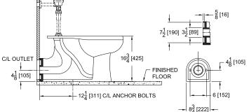
Rough-in/Overview dimensions for Z5640 Series Z5640-BWL with top spud Z5641-BWL with top spud and bedpan lugs
