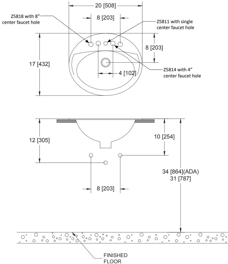
Fixture dimensions meet ASME A112.19.1 / CSA B45.2 requirements.
