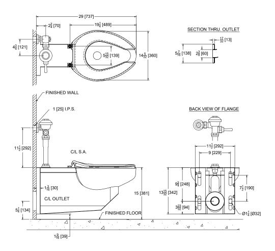
**Note:** For ADA compliance, rim height should be installed at 17"-19" from finished floor.
