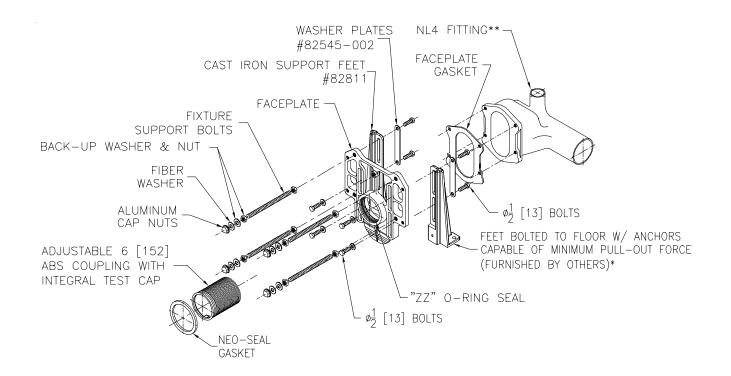
\*Carrier foot anchors must be able to withstand a pull-out force of 1004 Lb.[455 kg.]. Calculated value, no safety factor applied. \*\*Horizontal fitting shown. Vertical fittings also available.
