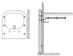
**3.** Gently slide lavatory onto the carrier arms to within 1/16" of the finished wall. The access holes on the underside of the lavatory should line up with the lockdown bar & adjustment screw holes of the arms.
