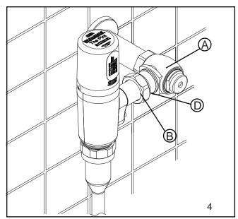
4.) Insert the flush valve tailpiece (B) into the stop valve (A) and hand tighten the lock nut (D) to the stop valve. Plumb the entire unit.
