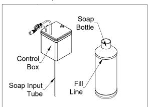
Re-attach the soap bottle to the control box, making sure that the soap input tube is inside the soap bottle.
