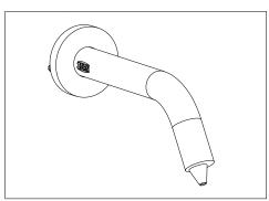
Note: It is recommended to horizontally offset the soap dispenser spout with the faucet 4 - 6" and to install vertically 6-10" above the sink drain at the same height as the faucet. To comply with ADA standards, the center-point of the soap dispenser spout must be less than 50" from finished floor.
