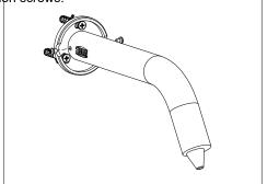
4. Reinstall the escutcheon by threading it clockwise onto the base.
