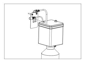
4. Push the soap tube onto the outlet connection on the control box. Secure the tube with the clamp.
