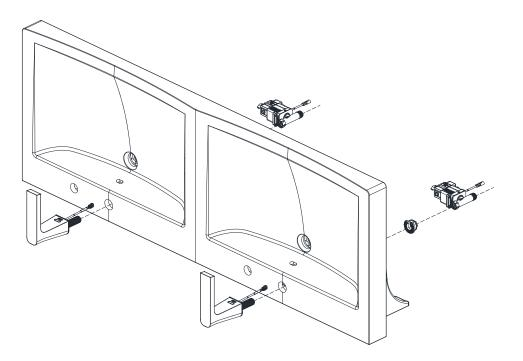
For ease of installion, lay basin on its back. Refer to faucet installation guide for details.
