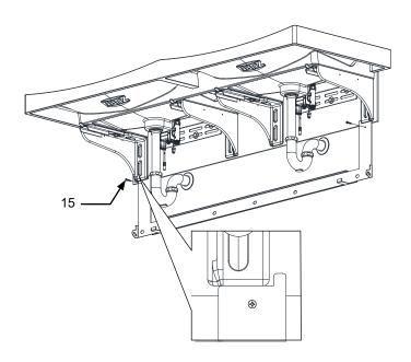
• Align wall bracket as shown and install coarse screw on each side. Mark the slots in the wall bracket on the wall.
