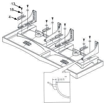
For ease of installion, lay basin on its top surface on a cushioned surface.
