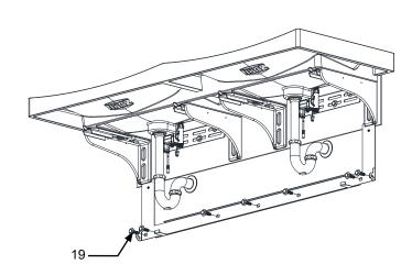
• Re-install wall bracket with coarse screws in previous location. Then, fasten the wall bracket with 3/8" bolts through each holes and into the toggle bolts.
