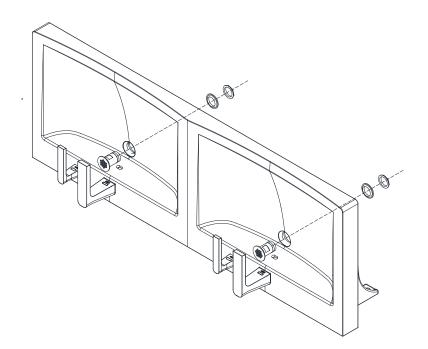
For ease of installion, lay basin on its back. Place grid drain into drainage opening. fasten washer and nut from underside of basin **Retrofitting Hanger Bracket** Installation
