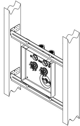
Step 3: Remove the paper backing from the gasket strip provided and adhere to the outer surface of the frame. Start from the top surface of the frame and wrap the gasket all around the frame. Make sure that the gasket is placed so that it is adjacent to the back corner of the frame cover (as shown in picture). Press firmly against the gasket to ensure that it makes sufficient adhesion with the frame.
