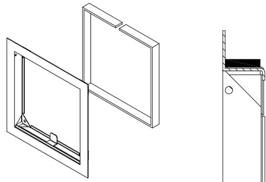
Step 4: Once the gasket is applied, make sure that the frame is oriented so that the hinged cover opens in an upward position. Slide the frame assembly into the hydrant box until the frame cover presses up against the finished wall surface.
