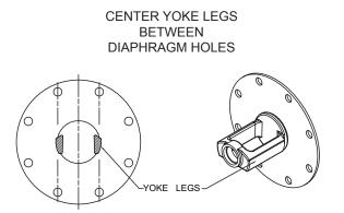
2. Next carefully slide yoke assembly into body and around pilot seat.
