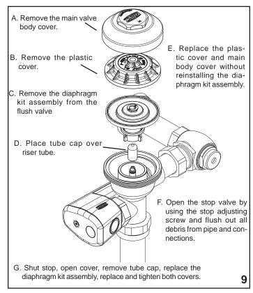
9. When all flush valves are connected to the fixtures and water pressure is available, it is recommended that the supply piping be flushed to remove dirt, pipe chips, etc., from system. This procedure should also be repeated when the system is drained for seasonal use, as occurs in athletic fields, recreation parks, etc.
