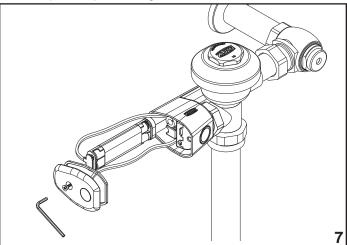
7. Remove electronics access cover with vandal-resistant hex wrench provided. Insert preassembled battery holder into electronics compartment. Connect battery cable connector to electronics cable connector. (Important: Insert non-connector end of battery holder first, as shown. Ensure foam spacer is in place)
