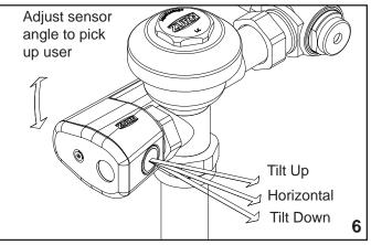
6. Loosen handle nut, aim sensor at desired tilt angle (horizontal, tilt up, or tilt down), hold in place and tighten handle nut
