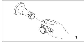
1. Install stop valve assembly using proper size supply escutcheon and sweat solder adapter kit if applicable. Thread sealing compounds should be used on male NPT threads only. Flush supply line by opening the control stop. Turn on water supply to flush line of any debris or sediment. Then close control stop.
