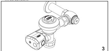
Insert the flush valve tailpiece into the stop valve and hand tighten the lock nut to the stop valve. Plumb the entire unit.
