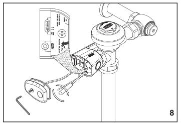
Adjust feature settings as desired. The sensor range is factory set. If adjustment is necessary, use a Phillips head screwdriver and turn GENTLY. SEE SENSOR RANGE ADJUSTMENT. Replace electronics access cover and tighten securely with vandal-resistant hex wrench.
