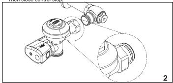
2. Prior to inserting the flush valve tailpiece into stop valve, be certain that the o-ring seal is located in o-ring seal groove at the end of the tailpiece and the locking nut and locking snap ring are located as shown. Care should be taken not to damage the o-ring when inserting the tailpiece into the stop valve. If lubrication is needed, wetting the o-ring with water will be sufficient.
