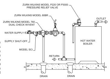
CAUTION: Anytime a reducing valve is adjusted, a pressure gauge must be used downstream to verify correct pressure setting. Do not bottom out adjustment bolt on bell housing. Valve may be installed in any position.
