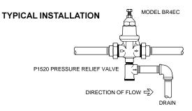
Regulators in series: Where the desired pressure reduction is more than a 4 to 1 ratio (i.e. 200psi to 50psi), multiple regulators in series should be installed.
