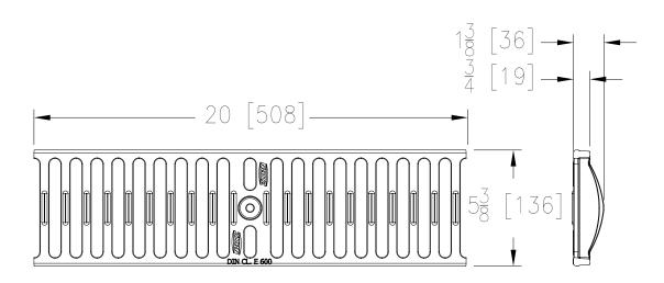
**GDE-USA GRATE ENGINEERING SPECIFICATION:** ZURN P6-GDE-USA 20" [508mm] X 5-3/8" [137mm] Galvanized ductile Iron slotted grate weighing 6.4 lbs per linear foot [9.5kg/m]. The grate has an open area of 28.2 in<sup>2</sup> per linear foot [597cm<sup>2</sup>/m]. Grate conforms to DIN rating of E, ANSI rating of Special-Duty, H-20 and FAA load rated, and ASTM A536 Grade 80-55-06. Galvanized (hot dip) conforms to ASTM A123.
