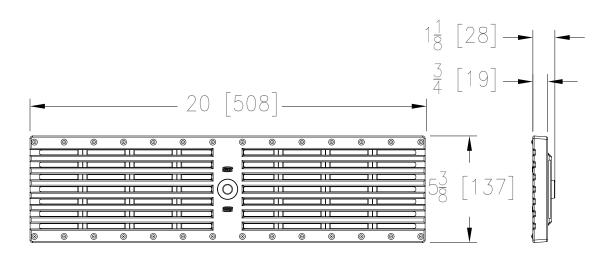
**HPP GRATE ENGINEERING SPECIFICATION:** ZURN P6-HPP 20" [508mm] X 5-3/8" [137mm] High Density Polyethylene (HDPE) heel-proof slotted grate weighing .9 lbs per linear foot [1.3kg/m]. The grate has an open area of 17.4 in<sup>2</sup> per linear foot [367cm<sup>2</sup>/m]. Grate conforms to DIN rating of A, ANSI rating of Light-Duty, ADA compliant\*, and Densetec 100 HDPE or Approved Equivalent.
