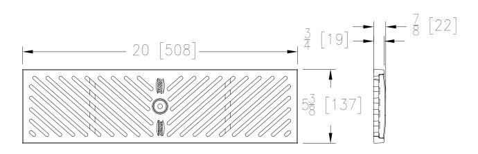
**DDD GRATE ENGINEERING SPECIFICATION:** ZURN P6-DDD 20" [508mm] X 5-3/8" [137mm] Ductile Iron diagonal decorative grate, weighing 5.5 lbs per linear foot [8.2kg/m]. The grate has an open area of 17.9 in<sup>2</sup> per linear foot [377cm<sup>2</sup>/m]. Grate conforms to DIN rating of A, ANSI rating of Light-Duty, ADA compliant and ASTM A536 Grade 80-55-06.
