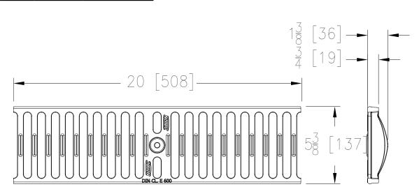
**BDE-USA GRATE ENGINEERING SPECIFICATION:** ZURN P6-BDE-USA 20" [508mm] X 5-3/8" [137mm] Black acid resistant epoxy coated Ductile Iron slotted grate weighing 6.4lbs per linear foot [9.5kg/m]. The grate has an open area of 28.2 in<sup>2</sup> per linear foot [594cm<sup>2</sup>/m]. Grate conforms to DIN rating of E, ANSI rating of Special-Duty, H-20 load rated, FAA load rated and ASTM A536 Grade 80-55-06.
