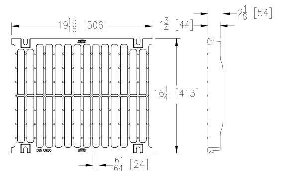
**GDC-USA GRATE ENGINEERING SPECIFICATION:** The Zurn P874-12-GDC-USA Slotted Grate, Galvanized Ductile Iron, is 16-1/4"[413mm] wide by 19-15/16"[506mm] long, weighing 28 lbs per linear foot[41.4 kg/m]. The grate has an open area of 118 square inches per linear foot[2497 cm²/m], DIN Rating of C, ANSI Rating of Heavy-Duty, H-20 Load Rated. Ductile Iron Conforms to ASTM Specification A536, Grade 80-55-06. Galvanizing (hot dip) conforms to ASTM specification A123.
