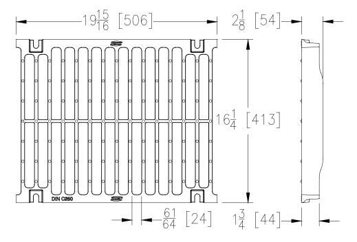
**DGC GRATE ENGINEERING SPECIFICATION:** The Zurn P874-12-DGC Slotted Grate, Ductile Iron, is 16-1/4" [413mm] wide by 19-15/16" [506mm] long, weighing 28 lbs per linear foot[41.4 kg/m]. The grate has an open area of 118 square inches per linear foot[2497 cm2/m], DIN Rating of C, ANSI Rating of Heavy-Duty, H-20 Load Rated. Ductile Iron Conforms to ASTM Specification A536, Grade 80-55-06.
