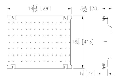
DCF COVER ENGINEERING SPECIFICATION: The Zurn P874-12-DCF Solid Cover, Ductile Iron, is 16-1/4" [413mm] wide by 19-15/16"[506mm] long, weighing 48 lbs per linear foot [71.4 kg/m]. The solid cover has a DIN Rating of F, ANSI Rating of Special-Duty, ADA Compliant, H-20 Load Rated and FAA Load Rated. Ductile Iron Conforms to ASTM Specification A536, Grade 80-55-06.
