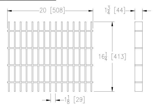
**SBG GRATE ENGINEERING SPECIFICATION:** The Zurn P874-12-SBG Slotted Bar Grate, Stainless Steel is 16-1/4"[413mm] wide by 20"[508mm] long weighing 24.17 lbs per linear foot[35.96 kg/m]. The grate has a open area of 143 square inches per linear foot [3027 cm2/m], DIN Rating of C, ANSI Rating of Heavy-Duty, Stainless Steel conforms to ASTM A-240 Type 304 (or Type 316 by request).
