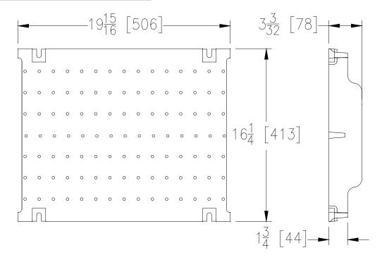
**GCF COVER ENGINEERING SPECIFICATION:** Zurn 16-1/4"[413mm] Wide by 19-15/16" [506mm] long Ductile Iron Galvanized Solid Cover. Ductile Iron conforms to ASTM specification A536, Grade 80-55-06. Ductile Iron Solid Cover is rated class F per the DIN 19580 top load classification. Four corner lockdown recesses provided for securing to frame. Galvanizing (Hot dip) conforms to ASTM specification A123.
