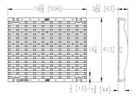
**ADA-USA GRATE ENGINEERING SPECIFICATION:** The Zurn P874-12-ADA-USA ADA Compliant, Ductile Iron Grate, is 16-1/4" [413mm] wide by 19-15/16"[506mm] long, weighing 26.5lbs per linear foot [39.4 kg/m]. The grate has an open area of 66 square inches per linear foot [1398 cm2/m], DIN Rating of C, ANSI Rating of Heavy-Duty, ADA compliant, H-20 Load Rated. Ductile Iron Conforms to ASTM Specification A536, Grade 80-55-06.
