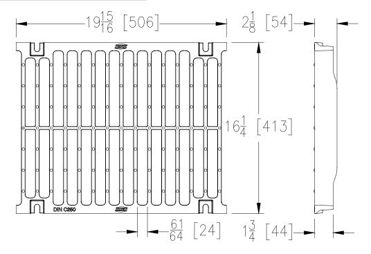
DGC-USA GRATE ENGINEERING SPECIFICATION: The Zurn P874-12-DGC-USA Slotted Grate, Ductile Iron, is 16-1/4" [413mm] wide by 19-15/16" [506mm] inches long, weighing 28 lbs per linear foot[41.4 kg/m]. The grate has an open area of 118 square inches per linear foot[2497 cm2/m], DIN Rating of C, ANSI Rating of Heavy-Duty, H-20 Load Rated. Ductile Iron Conforms to ASTM Specification A536, Grade 80-55-06.
