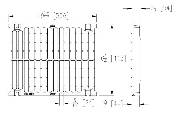
**GDC GRATE ENGINEERING SPECIFICATION:** The Zurn P874-12-GDC Slotted Grate, Galvanized Ductile Iron, is 16-1/4"[413mm] wide by 19-15/16"[506mm] long, weighing 28 lbs per linear foot [41.4 kg/m]. The grate has an open area of 118 square inches per linear foot [2497 cm2/m], DIN Rating of C, ANSI Rating of Heavy-Duty, H-20 Load Rated. Ductile Iron Conforms to ASTM Specification A536, Grade 80-55-06. Galvanizing (hot dip) conforms to ASTM specification A123.
