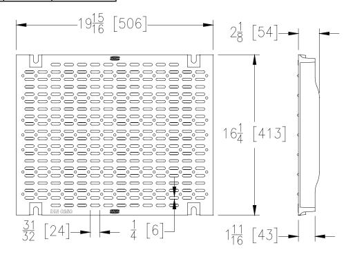
**HPD GRATE ENGINEERING SPECIFICATION:** The Zurn P874-12-HPD Heel-Proof Longitudinal, Ductile Iron Grate, is 16-1/4"[413mm] wide by 19-15/16"[506mm] long, weighing 28.5 lbs per linear foot[42.4 kg/m]. The grate has an open area of 37 square inches per linear foot[783 cm2/m], DIN Rating of C, ANSI Rating of Heavy-Duty, ADA compliant, H-20 Load Rated. Ductile Iron Conforms to ASTM Specification A536, Grade 80-55-06
