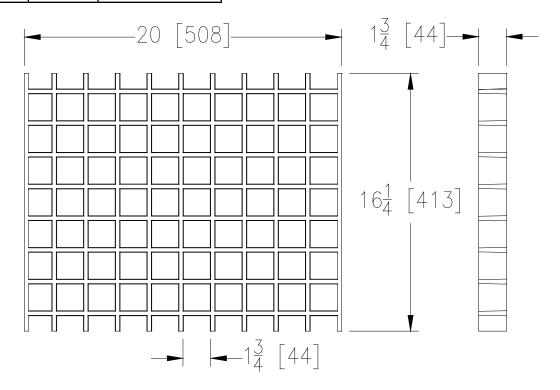
**GG GRATE ENGINEERING SPECIFICATION:** The Zurn P874-12-GG Fiberglass Grate, is 16-1/4"[413mm] wide by 20"[508mm] long, weighing 6 lbs per linear foot[8.9 kg/m]. The grate has an open area of 147 square inches per linear foot[3111 cm2/m], DIN Rating of A, ANSI Rating of Light-Duty. Fiberglass Conforms to Composition Resin Reich hold 31-509-01, glass NICO.
