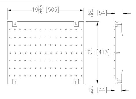
**DCC COVER ENGINEERING SPECIFICATION:** The Zurn P874-12-DCC Solid Cover, Ductile Iron, is 16-1/4"[413mm] wide by 19-15/16"[506mm] long, weighing 29 lbs per linear foot [43.2 kg/m]. The solid cover has a DIN Rating of C, ANSI Rating of Heavy-Duty, ADA Compliant, H-20 Load Rated. Ductile Iron Conforms to ASTM Specification A536, Grade 80-55-06.
