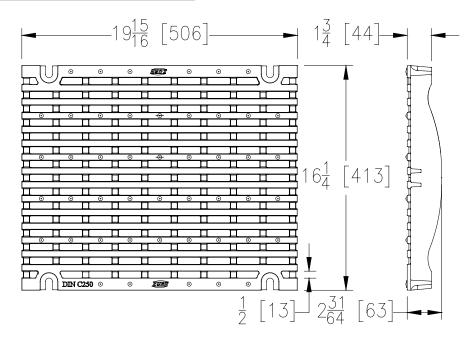
GADA-USA GRATE ENGINEERING SPECIFICATION: The Zurn P874-12-GADA-USA ADA Compliant, Galvanized Ductile Iron Grate, is 16-1/4"[413mm] wide by 19-15/16"[506mm] long, weighing 26.5 lbs per linear foot[39.4 kg/m]. The grate has an open area of 66 square inches per linear foot[1398 cm2/m], DIN Rating of C, ANSI Rating of Heavy-Duty, ADA compliant, H-20 Load Rated. Ductile Iron Conforms to ASTM Specification A536, Grade 80-55-06. Galvanizing (hot dip) conforms to ASTM specification A123.
