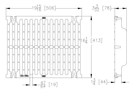
**GDF GRATE ENGINEERING SPECIFICATION:** The Zurn P874-12-GDF Slotted Grate, Galvanized Ductile Iron, is 16-1/4"[413mm] wide by 19-15/16"[506mm] long, weighing 49 lbs per linear foot [72.2 kg/m]. The grate has an open area of 90 square inches per linear foot [1902 cm2/m], DIN Rating of F, ANSI Rating of Special-Duty, H-20 Load Rated, FAA Load Rated. Ductile Iron Conforms to ASTM Specification A536, Grade 80-55-06. Galvanizing (hot dip) conforms to ASTM specification A123.
