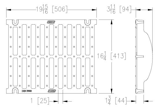
GDF-USA GRATE ENGINEERING SPECIFICATION: The Zurn P874-12-GDF-USA Slotted Grate, Galvanized Ductile Iron, is 16-1/4"[413mm] wide by 19-15/16"[506mm] long, weighing 39.8 lbs per linear foot [59.2 kg/m]. The grate has an open area of 120 square inches per linear foot [2540 cm2/m], DIN Rating of F, ANSI Rating of Special-Duty, H-20 Load Rated, FAA Load Rated. Ductile Iron Conforms to ASTM Specification A536, Grade 80-55-06. Galvanizing (hot dip) conforms to ASTM specification A123.
