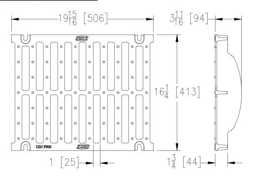
**DGF-USA GRATE ENGINEERING SPECIFICATION:** The Zurn P874-12-DGF-USA Slotted Grate, Ductile Iron, is 16-1/4" [413mm] wide by 19-15/16"[506mm] long, weighing 39.8 lbs per linear foot [59.2 kg/m]. The grate has an open area of 120 square inches per linear foot[2540 cm2/m], DIN Rating of F, ANSI Rating of Special-Duty, H-20 Load Rated, FAA Load Rated. Ductile Iron Conforms to ASTM Specification A536, Grade 80-55-06.
