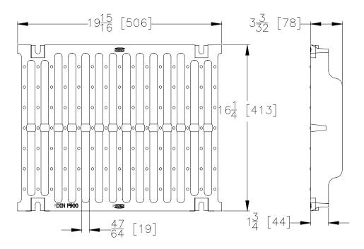
**DGF GRATE ENGINEERING SPECIFICATION:** The Zurn P874-12-DGF Slotted Grate, Ductile Iron, is 16-1/4"[413mm] wide by 19-15/16"[506mm] long, weighing 49 lbs per linear foot[72.2 kg/m]. The grate has an open area of 90 square inches per linear foot[1902 cm2/m], DIN Rating of F, ANSI Rating of Special-Duty, H-20 Load Rated, FAA Load Rated. Ductile Iron Conforms to ASTM Specification A536, Grade 80-55-06.
