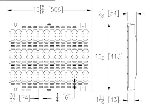
GHPD GRATE ENGINEERING SPECIFICATION: The Zurn P874-12-GHPD Heel-Proof Longitudinal, Ductile Iron Grate, is 16-1/4"[413mm] wide by 19-15/16"[506mm] long, weighing 28.5 lbs per linear foot [42.4 kg/m]. The grate has an open area of 37 square inches per linear foot [783 cm2/m], DIN Rating of C, ANSI Rating of Heavy-Duty, ADA compliant, H-20 Load Rated. Ductile Iron Conforms to ASTM Specification A536, Grade 80-55-06. Galvinized (Hot Dip) conforms to ASTM Specification A123
