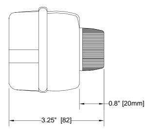
**Engineering Specification**: Zurn Four Way Mixing Valve Motor. The QHMVM56 provides motorized automatic mixing valve operation when used in conjunction with mixing controls. Reversible motor with fixed limit switches and optional contacts for independent control circuit switches. Start/stop of pump when limit position is reached.
