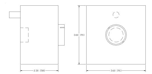
**Engineering Specification:** Zurn Snow Melt Switch allowing for the on/off control of a circulator pump. The 24VAC switch has a 2.5W maximum power consumption. The heated sensing grid detects moisture and closes a relay for a fixed 5 hours after the sensor has dried. The switch activates when the outdoor air temperature drops below 38°F (3.3°C). The snow switch has 1/2" FNPT mounting hole on the bottom.
