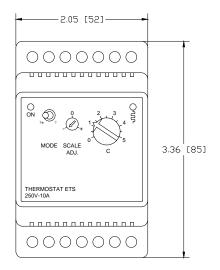
Engineering Specification: Zurn Snow Melt Thermostat for controlling a snow melt system. This 24VAC thermostat has a green power indicator LED and a red 'heating on' LED. The thermostat receives a signal from a sensor (QHGS) and powers a relay. The thermostat has a field selectable switch to sense temperature or temperature and moisture. The unit has a selectable temperature setpoint. The temperature range is 32°-41°F (0°-5°C). DIN rail mountable.
