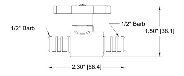
**Engineering Specification**: Zurn PEX<sup>®</sup> XL-Low Lead Brass Quarter-Turn Straight Stop Valve. The QQTV477GX has a 1/2" PEX barb inlet x 1/2" PEX barb outlet. Manufactured from EcoBrass<sup>®</sup>, C69300. These fittings, as a system with Zurn PEX<sup>®</sup> tube, are pressure rated at 160 PSI at 73°F, 100 PSI at 180°F, and 80 PSI at 200°F. These fittings are listed as complying with the following standards: NSF/ANSI Standard 61 including Annex G, CSA B137.5, and ASTM F1807.
