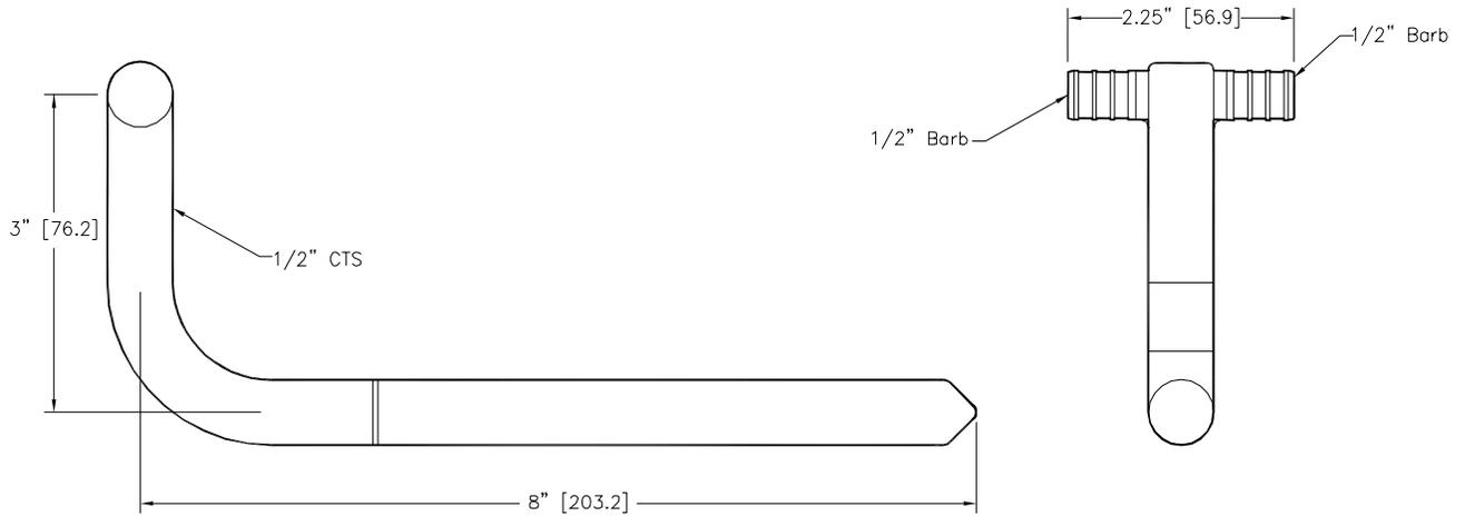
**Engineering Specification:** ZurnPEX<sup>®</sup> 1/2" Copper Stubout Tee Elbow. The QSTUBLXXT3 elbow tee is used in conjunction with PEX tubing. QSTUBLXXT3 is ideal for stubouts off of 1/2" ZurnPEX<sup>®</sup> runs. End spun closed allows for system testing before valves or other fittings are installed. Meets NSF<sup>®</sup> and ASTM requirements.
