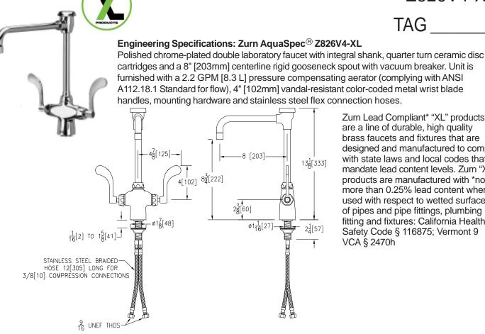
Zurn Lead Compliant\* "XL" products are a line of durable, high quality brass faucets and fixtures that are designed and manufactured to comply with state laws and local codes that mandate lead content levels. Zurn "XL" products are manufactured with \*not
