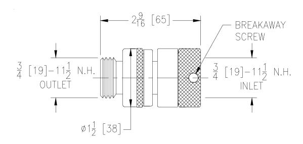
**ENGINEERING SPECIFICATION:** Z1399-BFP Backflow Preventer. Non-removable hose connection backflow preventer, field testable with dual independent backchecks, atmospheric vent, all brass construction, breakaway screw, and 3/4 [19] hose connection inlet/outlet.
