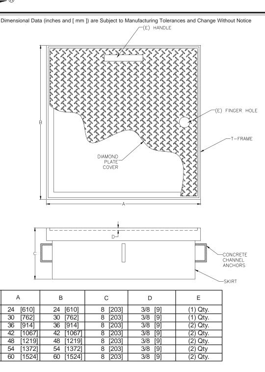
ENGINEERING SPECIFICATION: ZURN Z9-MAC Protective coated 14 Ga. steel skirt and 3/8 [9] diamond plate cover with a H-20 truck load rating manhole and cover assembly.
