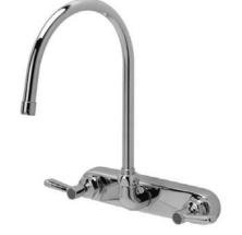
Engineering Specifications: Zurn AquaSpec® Z871C1-TWM-15F Wall mounted polished chrome-plated 8" [203mm] brass faucet with an 8" [203mm] centerline rigid or swing gooseneck spout and quarter turn ceramic disc cartridges. Unit is furnished with a full flow outlet, 2-1/2" [64mm] vandal-resistant color-coded metal lever handles and mounting hardware.
