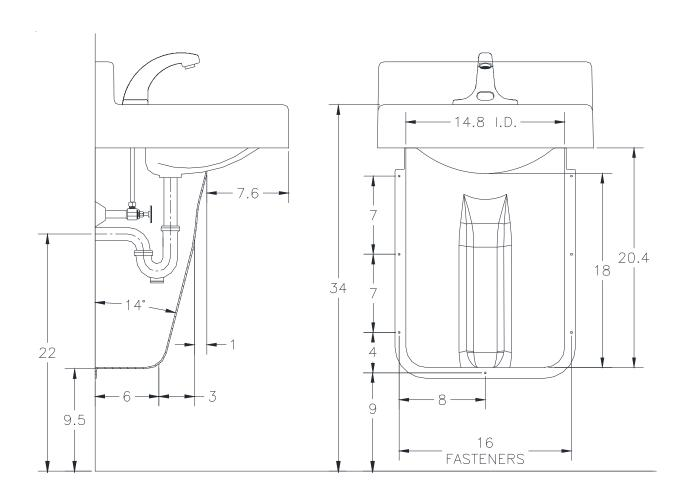
**Engineering Specification:** Zurn Z6900-VG - Rigid plastic lavatory enclosure for 20"[508mm] X 18"[457mm] lavatory. Conceals all lavatory piping, electronic faucet connection mixing valves, trap primers and instantaneous hot water heaters.
