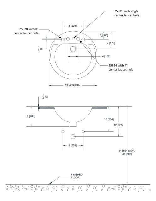
Fixture dimensions meet ASME A112.19.1 / CSA B45.2 requirements.
