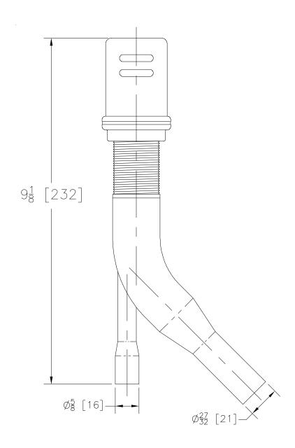
CD3P SPEEDFLEX AIR GAP - Copper with chrome cap
