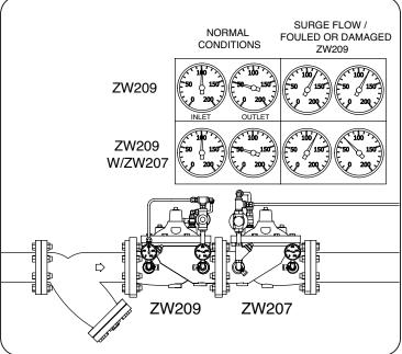
Caution: The recommended installation orientation for ACVs is horizontal, with the valve cover up. 6" and larger valves should only be installed horizontally, with the valve cover up, due to the difficulty of properly bleeding air out of the cover and performing maintenance on valves installed in the vertical orientation.
