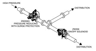
**Caution:** The recommended installation orientation for ACVs is horizontal, with the valve cover up. 6" and larger valves should only be installed horizontally, with the valve cover up, due to the difficulty of properly bleeding air out of the cover and performing maintenance on valves installed in the vertical orientation.
