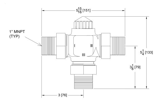
**Engineering Specification:** Zurn® 3-Way Diverter Valve. 1" Brass Valve, provides 0 - 100% by-pass. Has 1" union type male threaded connections. Operates manually or can be used with Zone Valve Actuators, Zone Valve Motors or Thermostatic Heads. Cv = 6.14.
