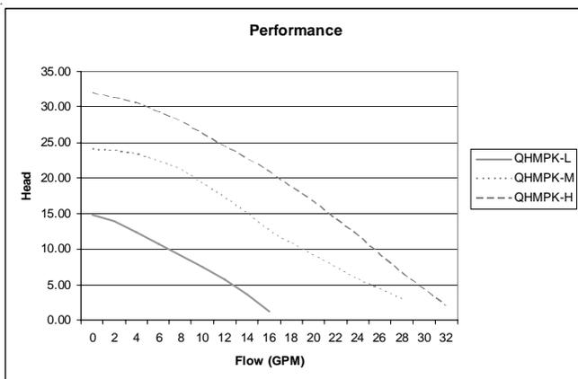
**Head Loss (FT-H2O) at Specified Flow Rate per Pump Size**
