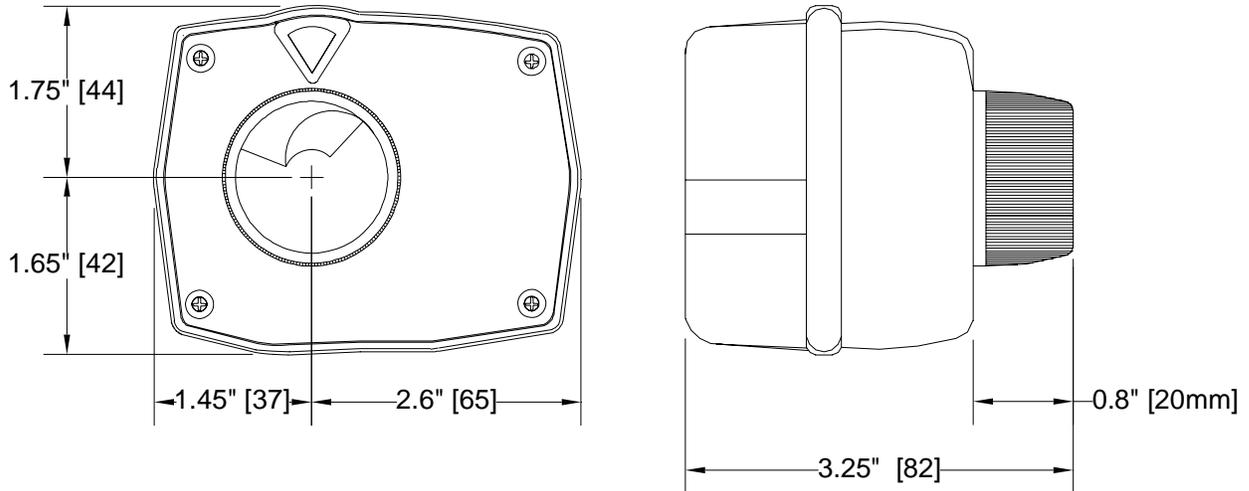
**Engineering Specification:** Zurn Four Way Mixing Valve Motor. The QHMVM56 provides motorized automatic mixing valve operation when used in conjunction with mixing controls. Reversible motor with fixed limit switches and optional contacts for independent control circuit switches. Start/stop of pump when limit position is reached.
