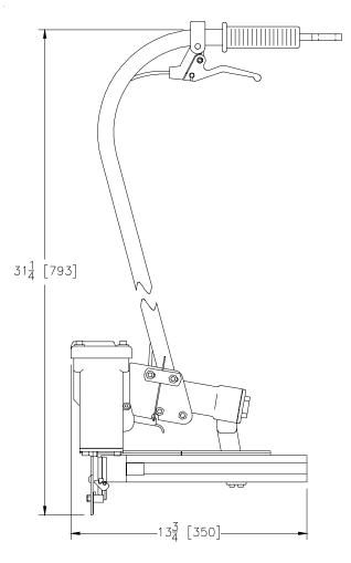
**Engineering Specification:** Zurn Pneumatic Staple Gun. Pneumatic staple gun with upright handle and tubing aligner used to attach ZurnPEX® to wood. Operates with 60 -100 PSI incoming air pressure.
