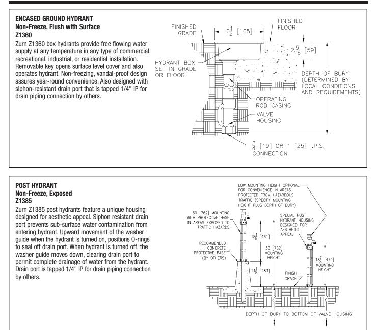
**NOTE:** For ground, post, and yard hydrant installations that involve the use of a drain port, it is recommended that gravel be placed around the drain port to allow a flow path for the drained water to evacuate.
